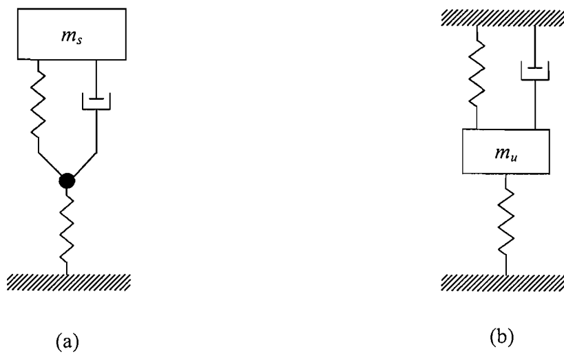
Figure 3.12: Approximation of bounce and wheel hop modes. (a) Bounce mode (b) Wheel hop mode.
