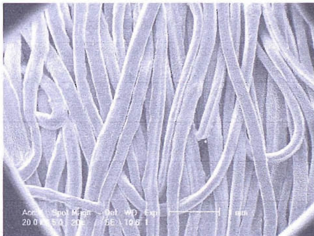
Figure 3.8.5 – Meltspun fibre mesh consisting of three layers using the structure A. These have been compressed to 100 kN.
