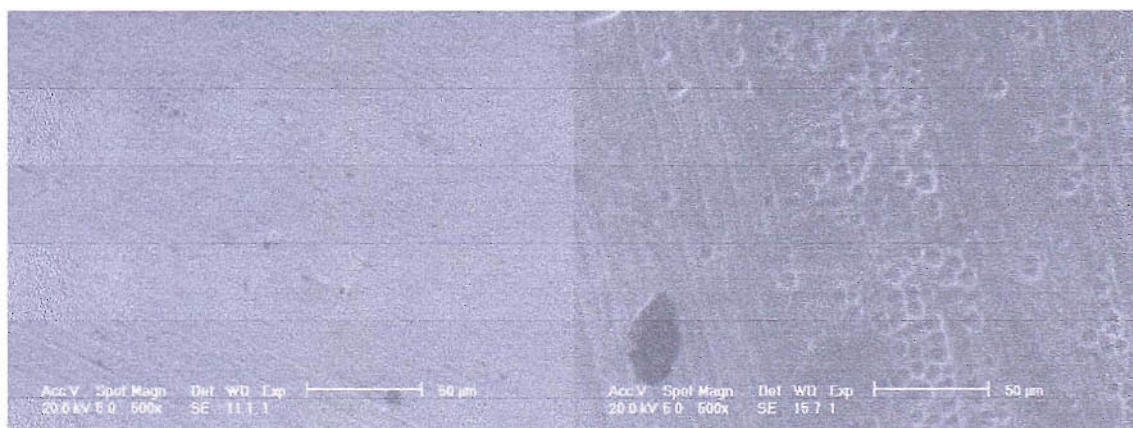
Figure 3.1.1 – SEM data of the surface of a high purity aluminium wire before/after submersion in 8M KOH for 1 hour at a temperature \sim 294\text{K} .
