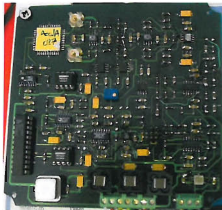
FIGURE 7.19: PCB of a fifth-order electromechanical \Sigma\Delta M.
