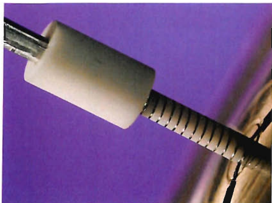
Fig 3.13 Macor collar surrounding heater
