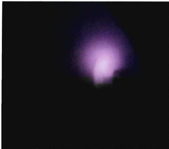
Fig 5.35 Erosion has caused discharge to couple to chamber wall
