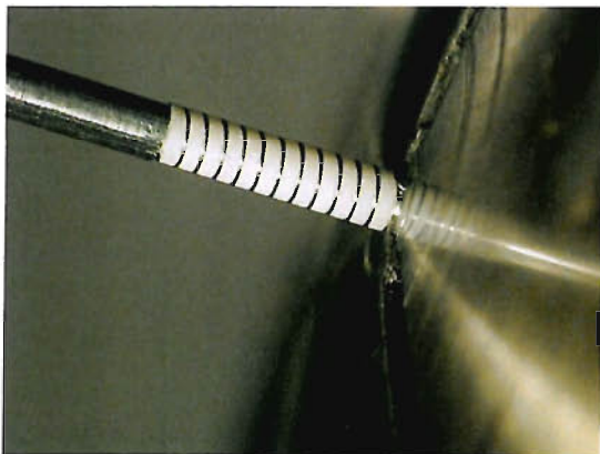
Fig 3.11 Shapal-M ceramic on mandrel
