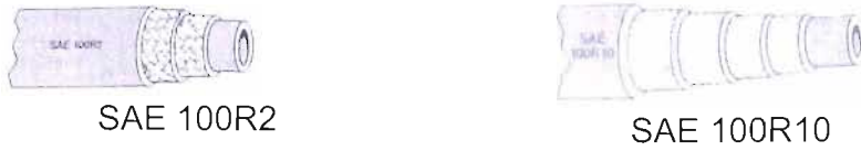
FIGURE 9.2: Fluid power hose used in the rig: SAE 100R2 was used in the previous design and it was replaced by SAE 100R10 to prevent excessive hose expansion.
