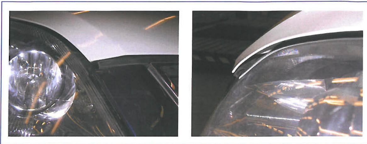
Figure 7.4 The Effect of Spring back on the Fit of the Closure to a Vehicle
