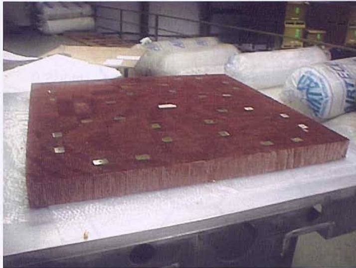
Figure 4.8: The NOMEX mask support structure to be attached directly underneath the IBIS coded mask.
