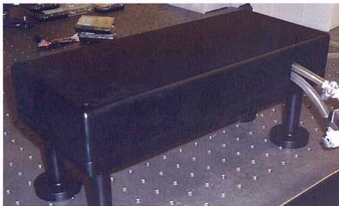
(b) A photograph of the complete laser, with its lid in place, making it stable, isolated from air movements, vibrations and temperature variations.
