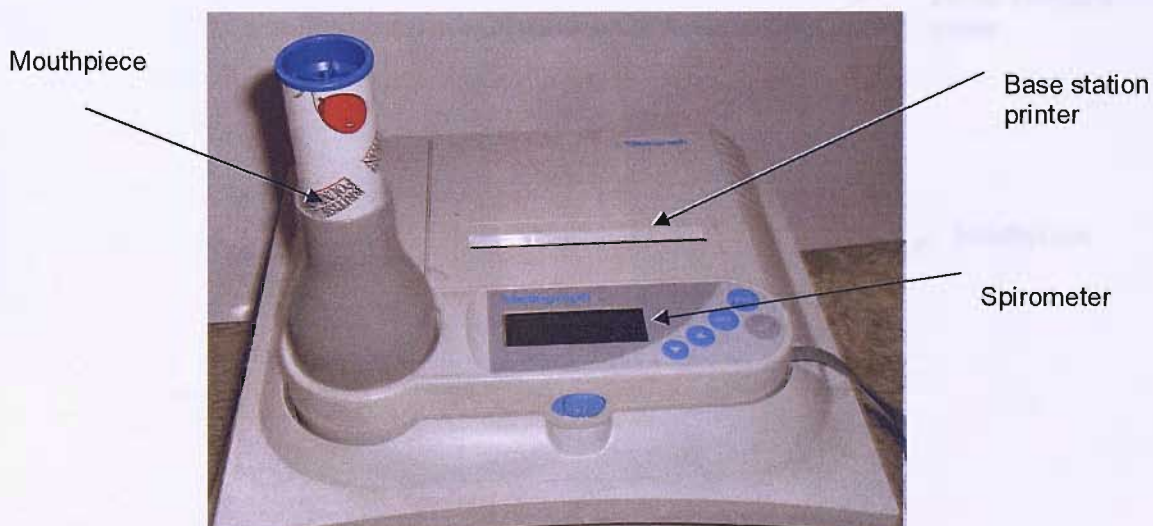
Figure 1.02: portable spirometry system with base station printer
