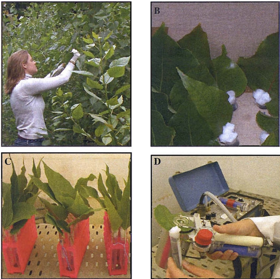
Figure 2.7 Sampling and measurement of stomatal conductance in Family 331. A) Leaf selection and sampling, B) Leaf transportation, C) Leaf acclimatization in D) Leaf conductance measurement using Licor 1600
