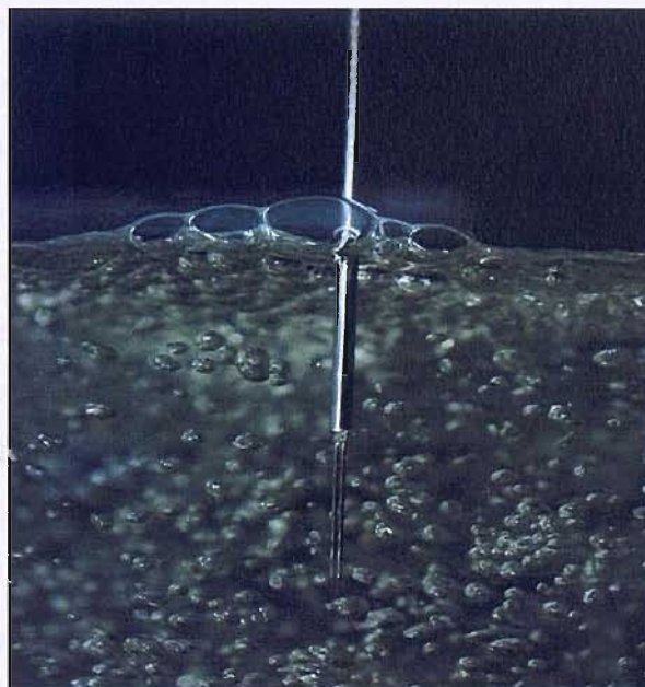
Figure 3.7 Double-tipped optical fibre phase detection probe.
