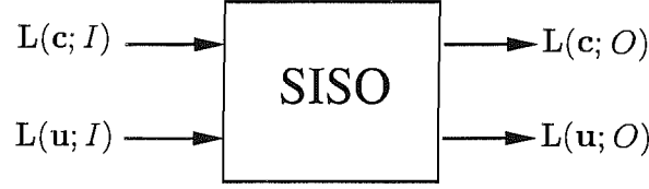
Figure 3.7: A SISO module operating in the log-domain.
