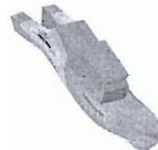
Figure 8.12: 3-node vertical(28.350 Hz)
