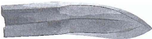
Figure 8.11: mode coupling(27.375 Hz)
