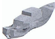
Figure 8.14: 4-node vertical(33.483 Hz)
