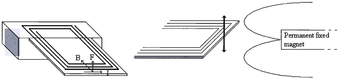
Figure 4.3: Electro-magnetic actuation, where \mathbf{B} is the constant magnetic field, I is the alternating current in the coil and \mathbf{F} is the force produced
