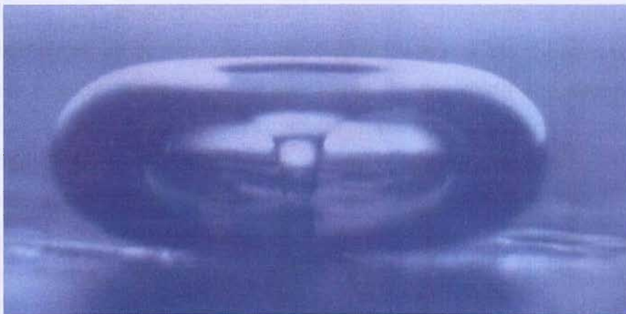
Figure 1.8 Jet formation during the collapse of an oscillating gas-vapour bubble at low pressure (0.04-0.05 bar) in a 60 Hz sound field. The bubble size is approximately 0.2 cm (published in reference [70]).
