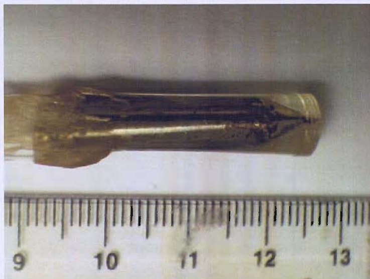
Figure 2.15 Photograph of the carbon steel microelectrode. The scale is in cm.
