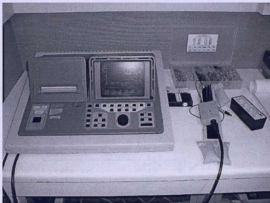
Figure 3.4: Tympanometer: measuring the compliance of the eardrum.
