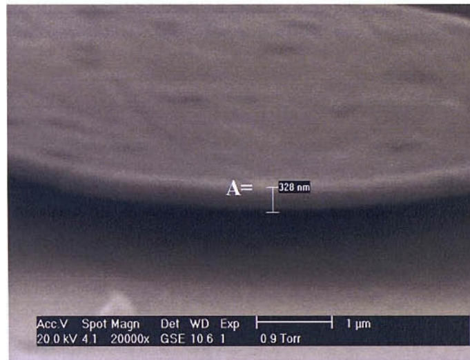
Figure 9.2 SEM photograph of a nanostructured Pt film edge. Marked on the photograph is the measured distance A (the shortest distance between the top edge of the film and the beam direction) used to estimate the film thickness.
