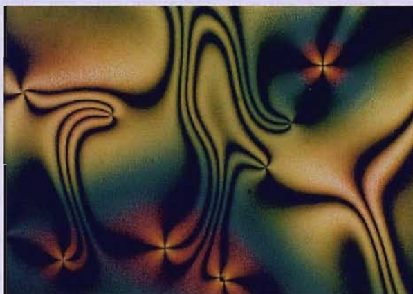
Figure 6 A Schlieren texture of a nematic film with four-brush defects [22].
