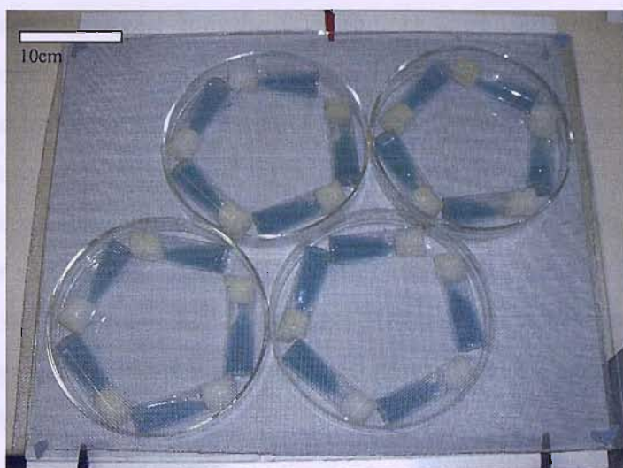
Figure 6.4 Photograph of fecundity setup. Each setup consisted of five vials within four glass dishes positioned on top of an earthed aluminium mesh. Another mesh, connected to the high voltage power supply, was placed on top of the dishes and covered with a glass sheet. Three identical setups tested the effect of electric field exposure during larval development on female fecundity, and exposure during adulthood on fecundity, in addition to controls.
