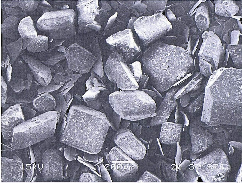
Figure 3.14. Scanning electron micrograph of castor sugar and mica particles
