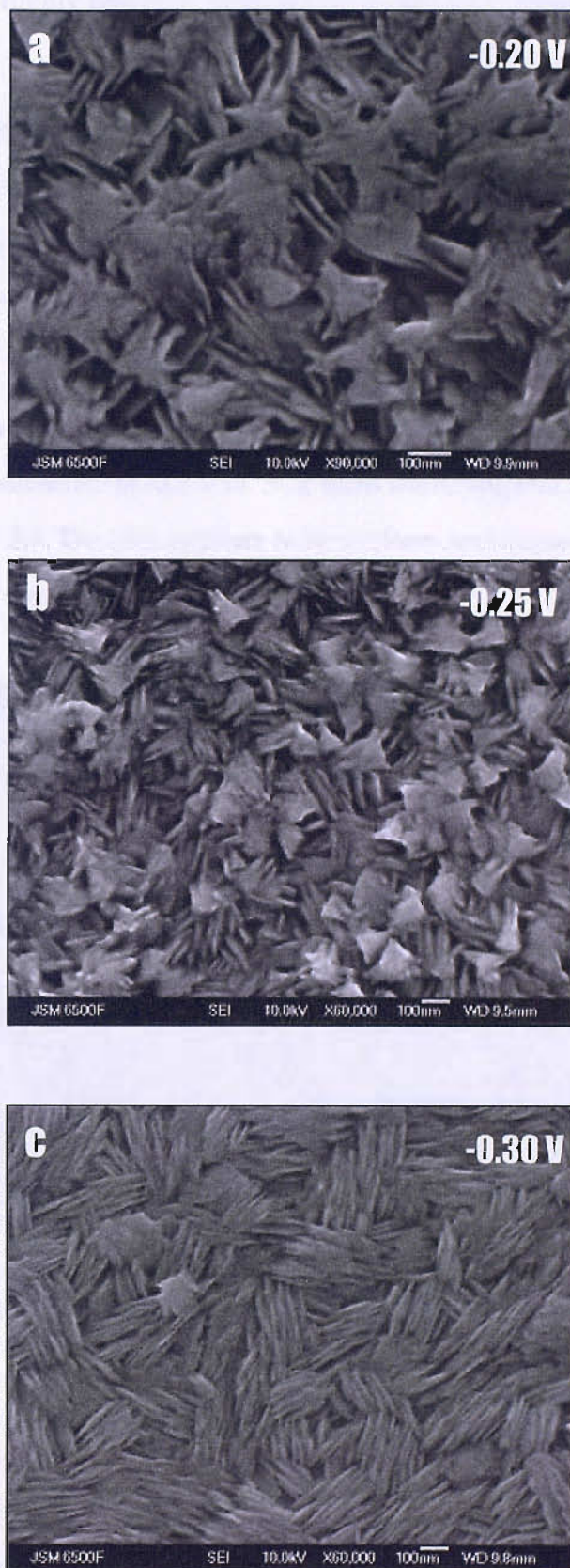
Figure 3.8: FE-SEM micrographs of Hi-eTe films electrodeposited at a). -0.2 V, b). -0.25 V and c). -0.3 V vs. SCE from a mixture containing 50 wt. % of a 5 mM \text{TeO}_2/2\text{M H}_2\text{SO}_4 solution and 50 wt. % \text{C}_{16}\text{EO}_8 . The charge density for the films was 0.82 \text{ C cm}^{-2} in all three cases.
