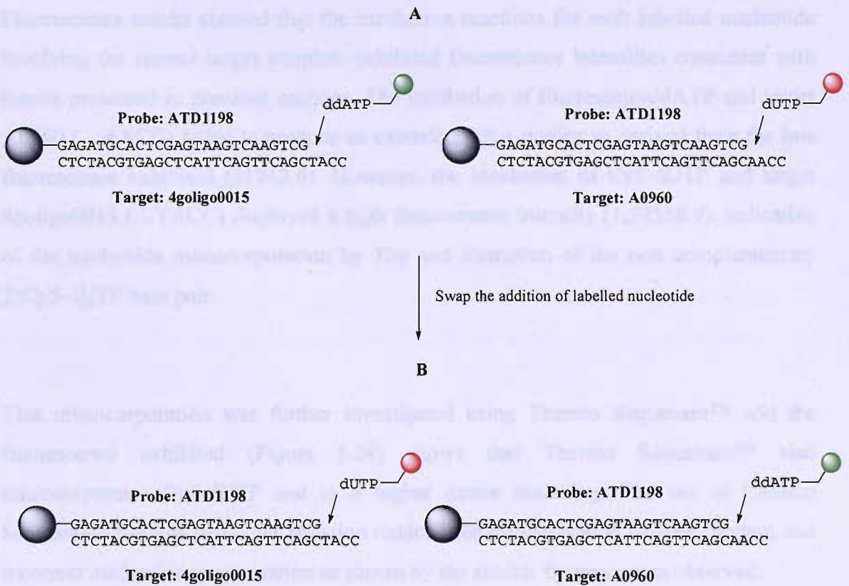
Figure 5.22 A- Oligonucleotide probe and targets sequences required for the respective base extensions and the indicated nucleotide incorporation site. B- Swapping the labelled nucleotides in the incubation samples.
