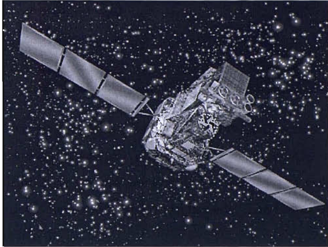
Figure 1.2: An artist's impression of the INTEGRAL spacecraft. At the front is the SPI instrument with its circular coded mask and behind the square mask of the IBIS instrument. JEM-X, the X-ray monitor, is located between these two instruments with the OMC (Optical Monitoring Camera) to the side. The INTEGRAL payload is described in detail in Section 3.
