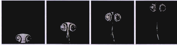
Figure 6.9: Dye visualization of the first moments of the evolution of a vortex ring at t=4s , 8s , 12s and 16s ; the Reynolds number is about 1000. The orifice at which the ring is created is located just below the bottom of each image; the height of each image is about 12 cm. Taken from http://www.fluid.tue.nl/WDY/vort/vortrings/vortrings.html .
