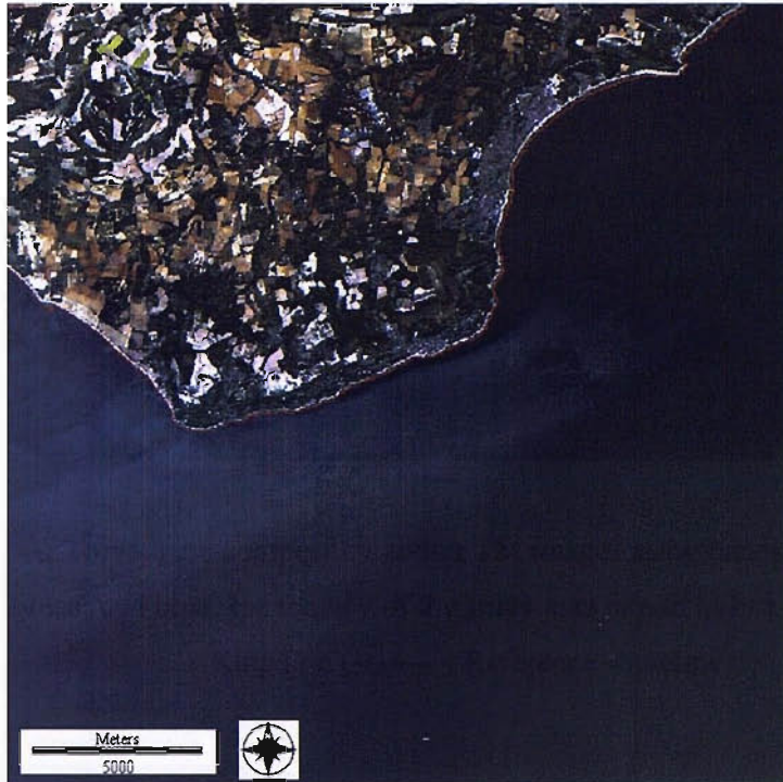
Figure 5.1: Three-band composite Landsat TM images using bands 3, 2, and 1 mapped to red, green, and blue respectively of the study area in part of Isle of Wight in United Kingdom (— : Reference shoreline).
