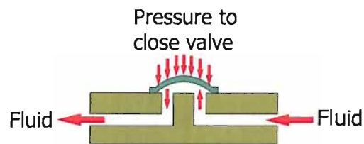
Figure 3.19: An illustration of a single fluid control valve.
