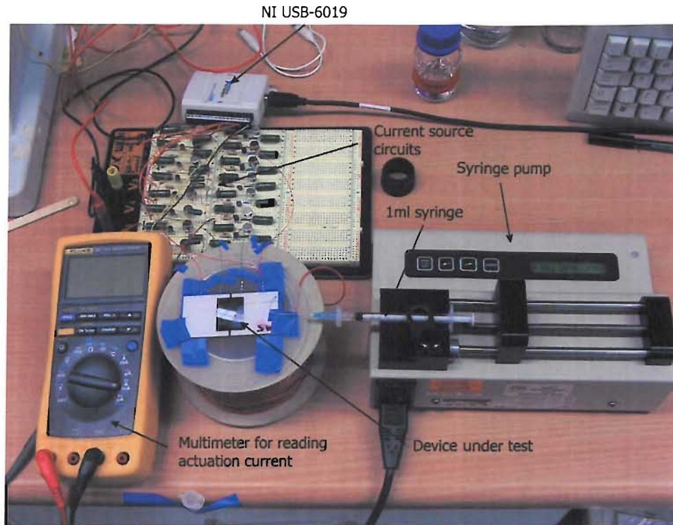
Figure 7.3: An image of the experimental set up used to investigate the integrated device operation.
