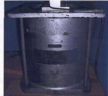
Figure 3-3 Exterior view of the VP4 vibrator with a metal plate and force cell on the top
