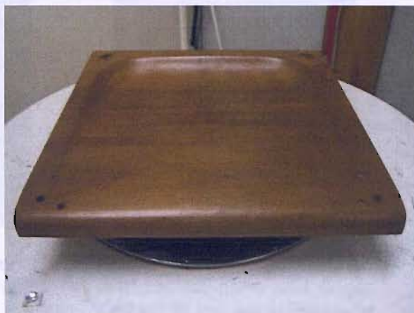
Figure 3-19 Wooden rigid seat used to contact buttocks with shaker in Experiment 3
