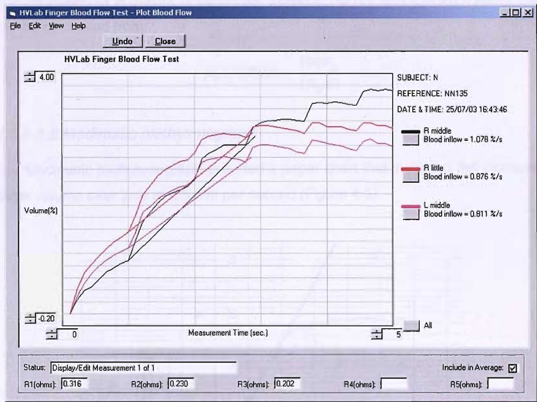
Figure 4-1 Change in strain recorded on five fingers following occlusion (60 mmHg occlusion pressure, 8-second occlusion duration)
