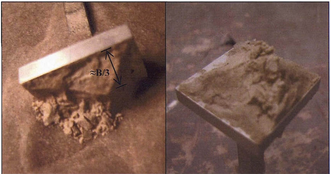
Figure 6.11 Wedge of clay adhered to anchor base after uplift ( v_f \geq 30 mm/s)
