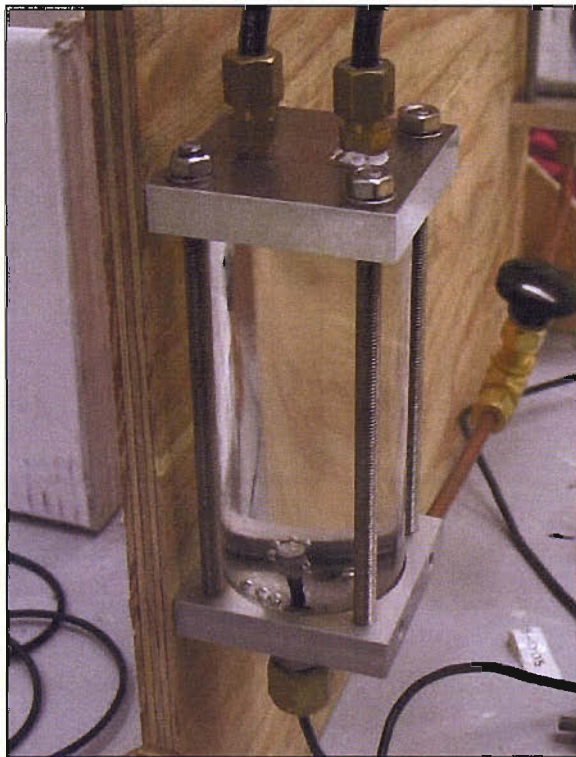
Figure 5.21 The PPTT during initial saturation under vacuum
