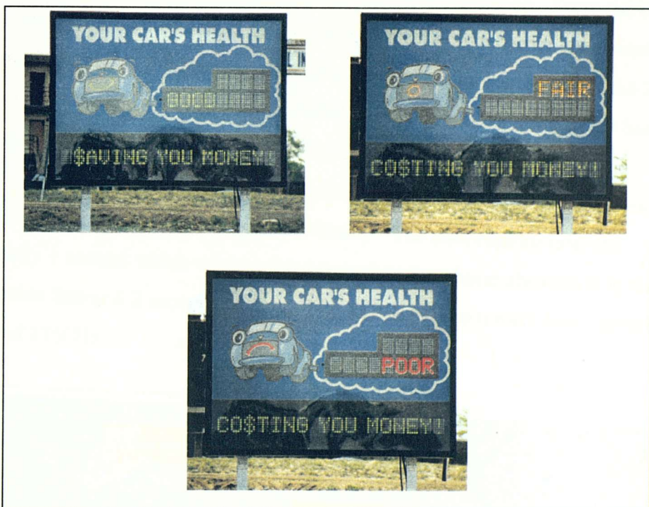
Figure 5-10: Smart Sign displaying showing three different levels of emissions and its relative financial implications (Source: Bishop et al., 2000 )
