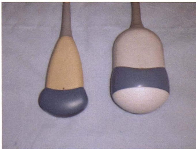
Figure 2.18: KretzGE transducers. Left: standard 2D transducer. Right: 3D transducer, which is larger to accommodate the mechanical sector sweep array.
