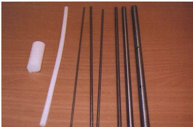
Figure 3.2: White Perspex and steel rods used in the test-tank. N.B. the variety of diameters.
