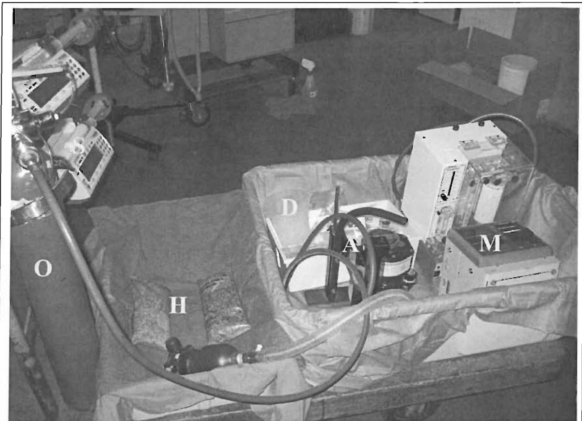
Figure 9.1 Animal transfer trolley, complete with portable oxygen (O), ventilator (V), anaesthetic machine (A), syringe drivers (S), heat pads (H), monitors (M), and emergency drugs (D).
