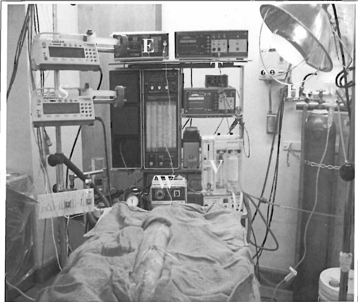
Figure 6.10 Laboratory intensive care set up. The piglet is managed in this fashion for 20hrs. This requires continuous supervision. The experiments therefore take 28hrs in total until completion. H = heat lamp, S = syringe drivers (propofol and noradrenaline), W=water blanket, V=ventilator, T=temperature monitors, E=end-tidal CO2 monitor.
