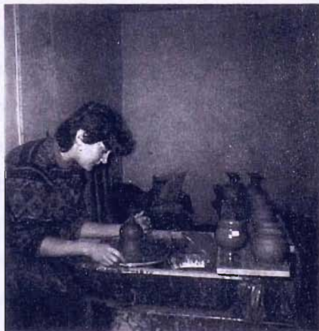
Figure 6.7 Production throwing at the author's workshop c. 1982. The wine goblet placed on the end of the 'throwing' board provides a visual template to allow standardisation
