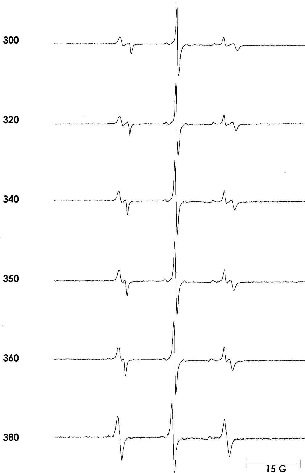
Figure 13: (a) ESR spectra for Tempone in chiral nematic ZLI-4792 doped with 0.5wt% cholesteryl propionate.
