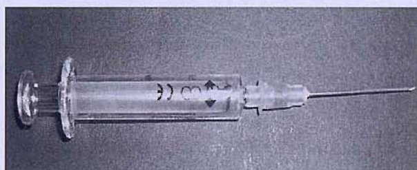
Figure 41: Syringe that was used to introduce the sample into the capillary tube. The size of needle can be important as it controls shear on nematic.
