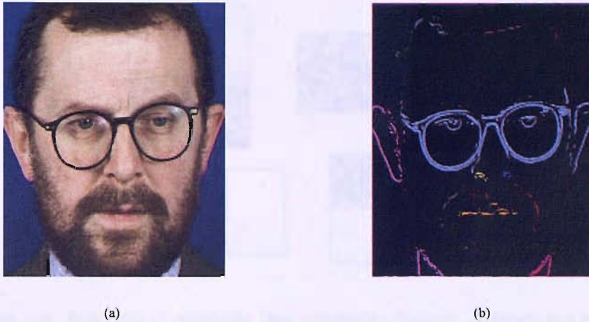
FIGURE 3.8: Another example in which the eye glasses link the two eyes together. (a) The original face image. (b) The blocks of the face image. Different blocks are represented by different colours.
