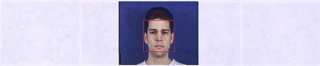
FIGURE 3.11: The face detection result generated by the AdaBoost algorithm. The face is represented by a red square.
