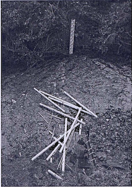
Figure 8.2 Dowels placed on a riffle at low flow at Site 3. For scale, the largest dowels are 1.06 m in length and 0.035 m in diameter.
