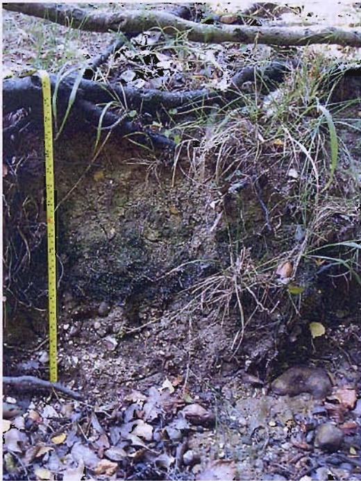
Figure 5.21 (a) Approximately 0.2 m; (b) Approximately 0.5 m of fine material above gravel in the floodplain.
