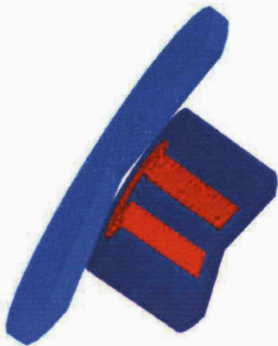
FIGURE 9.4: Coil, former and disc arrangement in Opera-3d.
