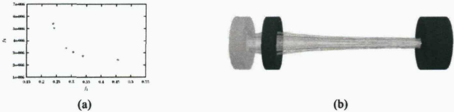
Fig.1 (a) Pareto optimal front for electron gun problem, and (b) the right-most Pareto-optimal solution (which has the most parallel beam, as measured by objective f_2 ), as found using algorithm X from Table 1.
