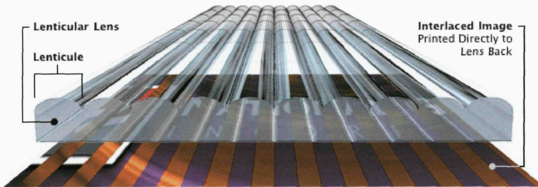
Fig. 16 A schematic representation of Interlaced Image
