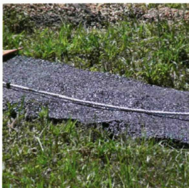
Figure 1.6 HIF on asphalt surface
