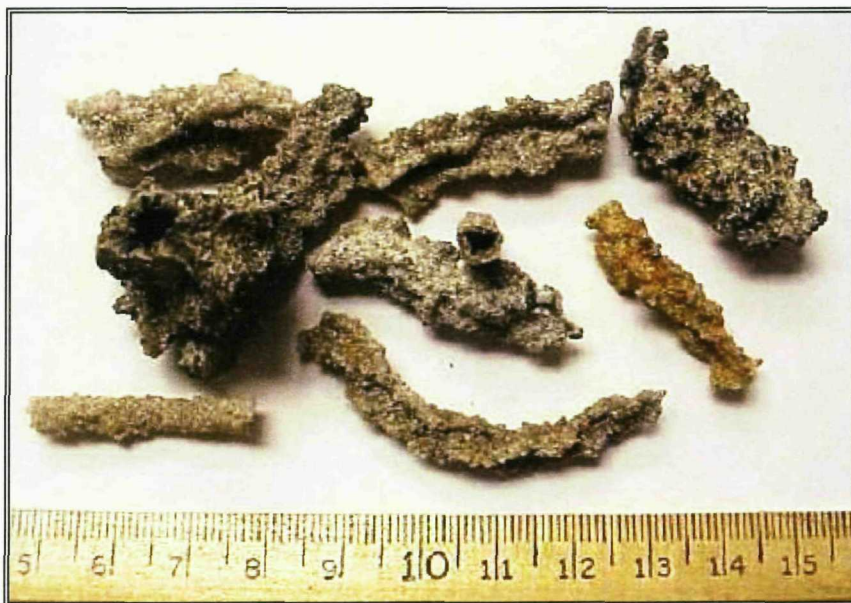
Figure 3.6 Molten material due to arcing creates a tube-like formation
