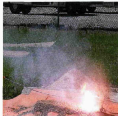
Figure 1.3 HIF on gravel surface
