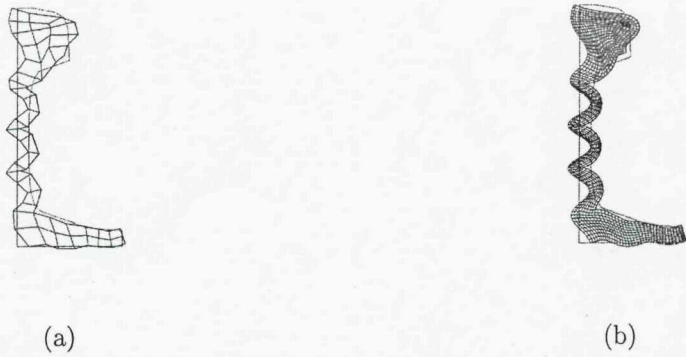
Fig. 3.4. Comparison of mode shapes at the 20th mode of the lateral and torsional modes for (a) model 1 (70.96 kHz), (b) model 3 (70.5 kHz).
