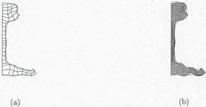
Fig. 3.3. Comparison of mode shapes at the 16th mode of the vertical modes for (a) model 1 (72.2 kHz), (b) model 3 (72.06 kHz).
