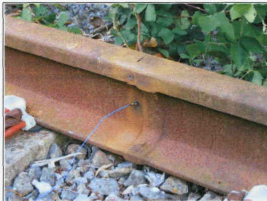
Fig. 6.4. A welded region located between 1st and 2nd measurement positions. An accelerometer can be seen attached at the 2nd measurement position on the web.
