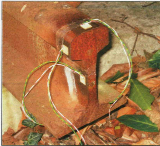
Fig. 6.32. Piezoceramic transducers attached at the top and side of the rail head and the middle of the web.
