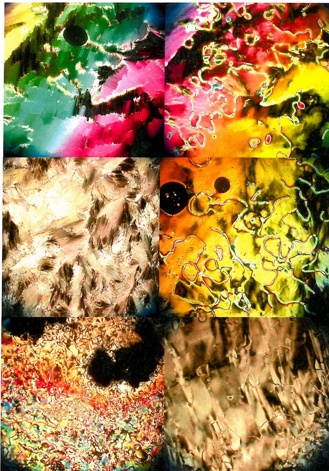
Figure 4.14 All optical textures are taken on cooling showing a smectic A (top left) and nematic (top right) from CBO8OPCH7 taken at 116 °C, 0.89 T_{NI} and 128 °C, 0.92 T_{NI} respectively; a smectic A (middle left) and nematic (middle right) from CBO9OPCH7 taken at 75 °C, 0.87 T_{NI} and 123 °C, 0.99 T_{NI} respectively; nematics for CBO10OPCH7 (bottom left) and CBO11OPCH7 (bottom right) at 144 °C, 0.92 T_{NI} and 133 °C, 1.02 T_{NI} respectively.
