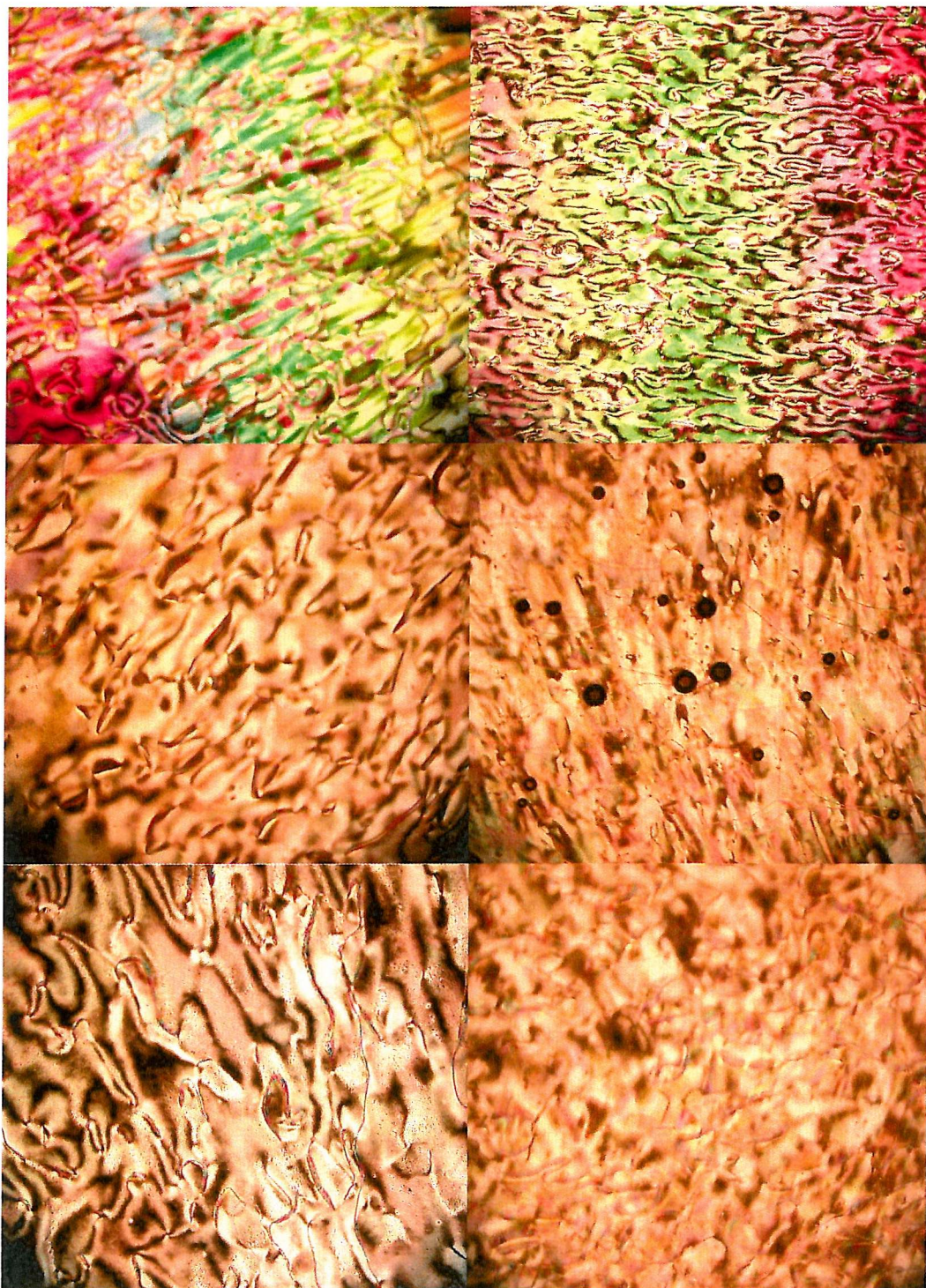
Figure 4.21 All optical texture pictures taken on cooling showing nematic phases. CBO6OCH3 130 °C, 0.95T_{NI} (top left); CBO7OCH3 taken at 133 °C, 1.15T_{NI} (top right); CBO8OCH3 taken at 127 °C, 0.99T_{NI} (middle left); CBO9OCH3 taken at 138 °C, 1.10T_{NI} (middle right); CBO10OCH3 taken at 166 °C, 1.09T_{NI} (bottom left); CBO11OCH3 taken at 135 °C, 1.09T_{NI} (bottom right).
