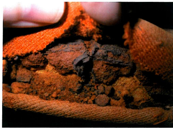
▲ Figure 84: A detail of a prototype (c. 1959) for the Cone chair by Vernor Panton showing hard, brittle, deformed foam. VDM – MPA-1152 (Photo – J. Wickens)
