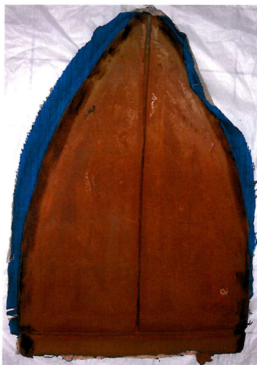
▲ Figure 40: The reverse of one of the pads donated by Michael Marks showing the reverse of the original blue top cover at the edges and the channels cut to accommodate the stabilizing bars. (Photo – J. Wickens)
