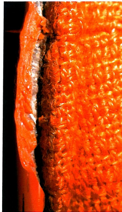
▲ Figure 48: A detail of the Ball chair in Figure 47 showing a cross-section of the gel coat(?) and fibreglass(?) shell. VDM - SSK-1002 (Photo – J. Wickens)
