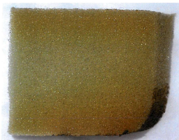
▲ Figure 66: A 5 cm by 4 cm cross-section of 2CM Pad 5 cut from the area beneath the still functional adhesive where the previously mentioned pH determinations were made. (Photo – J. Wickens)
