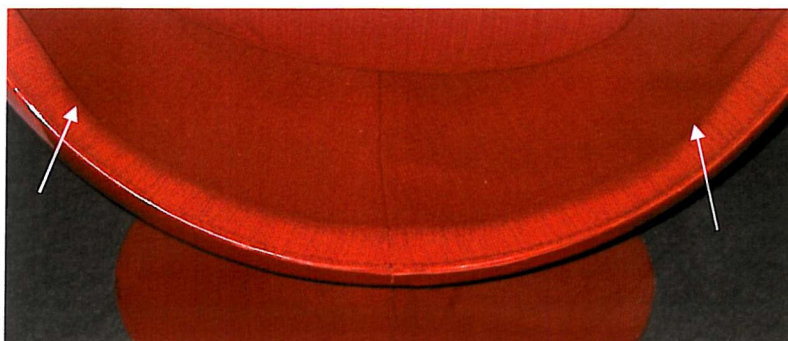
◀ Figure 58: The lower third of the Globe with the seat cushion removed. The tip of each arrow indicates the point where the compression in the shell pad foam is most visible. V & A – Circ. 12-1969 (Photo – J. Wickens)
