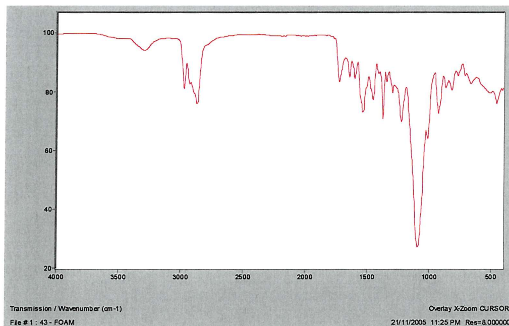
▲ Figure 138: A FTIR spectrum of a sample of foam removed from the pad at the centre of the loose back cushion of the Globe . Comparison with the spectrum in Figure 136 identifies it as polyether polyurethane foam.
