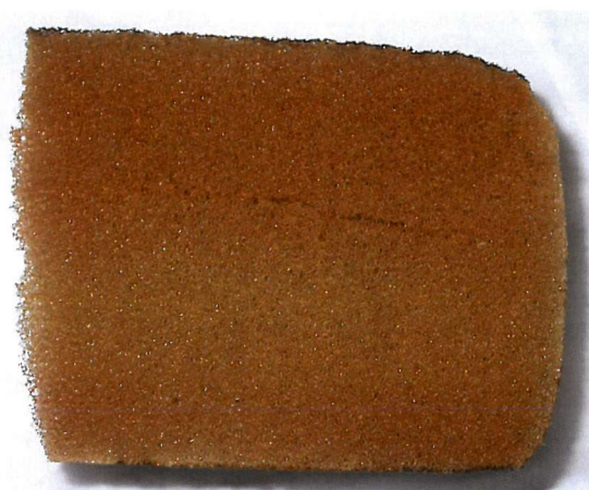
▲ Figure 67: A 5 cm by 4 cm cross-section of 2CM Pad 5 cut from the area beneath the no longer functional adhesive where the previously mentioned pH determinations were made. (Photo – J. Wickens)
