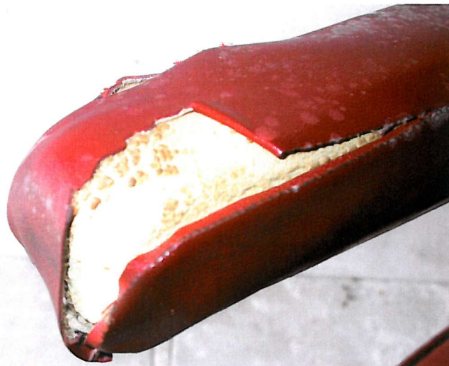
▲ Figure 8: A Ministry of Defence armchair, English Heritage collection in storage at Fort Brockhurst. Detail of proper right armrest in Figure 7 showing expanded foam. EH – no catalogue number (Photo – J. Wickens)
