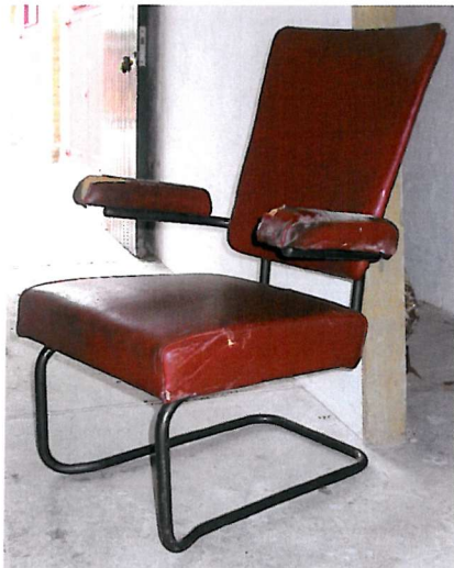
▲ Figure 7: A Ministry of Defence armchair, English Heritage collection in storage at Fort Brockhurst. The foam in the armrests is expanding and distorting the profile. EH – no catalogue number (Photo – J. Wickens)
