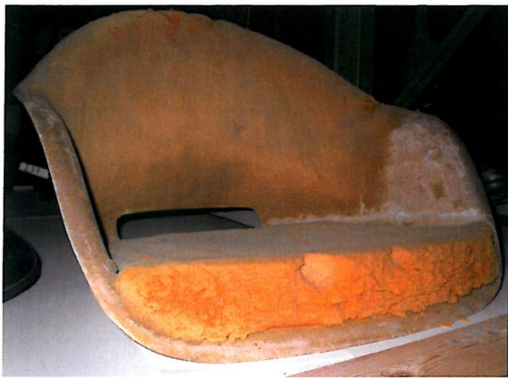
▲ Figure 83: A prototype for a chair by Charles Eames (date unknown) in which the foam is now severely degraded, crumbling. VDM – no catalogue number (Photo – J. Wickens)
