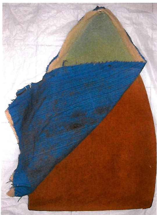
▲ Figure 39: The obverse of one of the pads donated by Michael Marks showing parts of the adhesive coated foam surface, the reverse of the original blue top cover and the obverse of a second green top cover. (Photo – J. Wickens)
