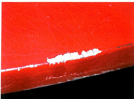
▲ Figure 55: Paint chips at the edge of the pedestal with barely visible fine cracking across most of the visible surface. V & A - Circ. 12-1969 (Photo – J. Wickens)
