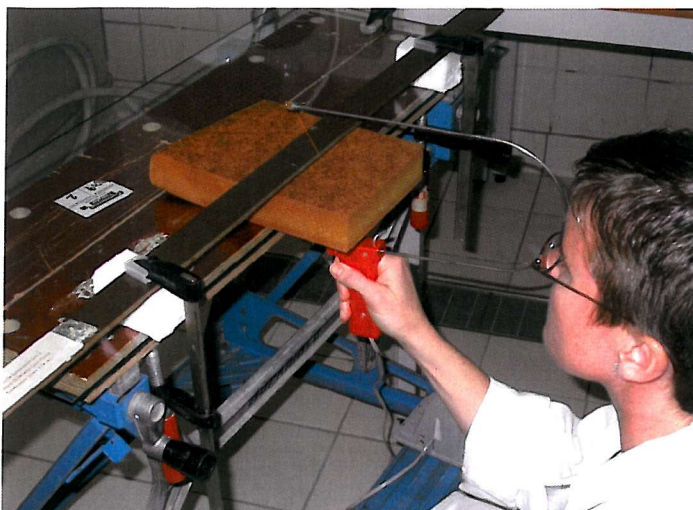
◀ Figure 96: A portion of one of the 2CM pads being cut to size with the Janik Pyrocutter. Straight edge guides have been placed in parallel above and beneath the foam and the glowing hot wire can just be seen pressing against the top straight edge as the wire cuts through the foam. (Photo – M. Halliwell)
