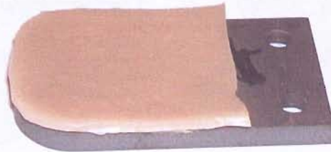
Figure 8.1: Prototype Fingertip with a tailored section of Otto Bock cosmetic glove adhered to the back.
