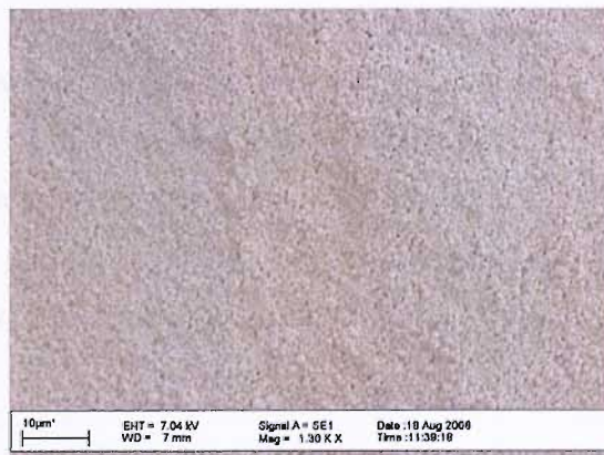
Figure 5.6: SEM micrograph of binderless piezoelectric thick-film cured at 150°C for 30 minutes in an IR drier.
