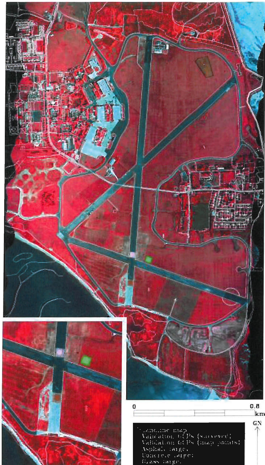
FIGURE 4.2: Figure showing an ATM false colour composite (Red: Band 7; Green: Band 5, Blue: Band 2) image of Thorney Island (collected 24th July 2001). The insert shows the primary study area in greater detail. The image is overlain with OS Land-Line.Plus data. Validation GCPs are also shown. Validation GCPs are gathered either from the Land-Line.Plus map or via surveying.
