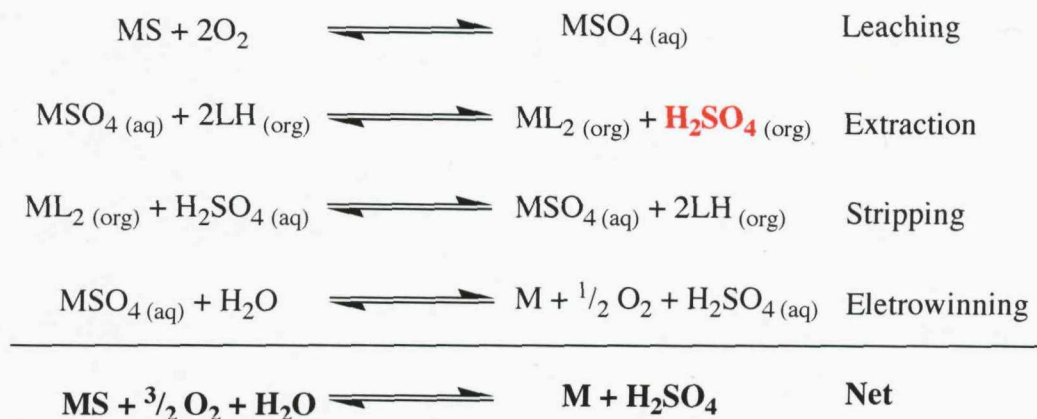
Figure 4.7: Material balance of phenolic oxime extraction of metals from sulfidic ores showing the generation of sulfuric acid during the extraction step.
