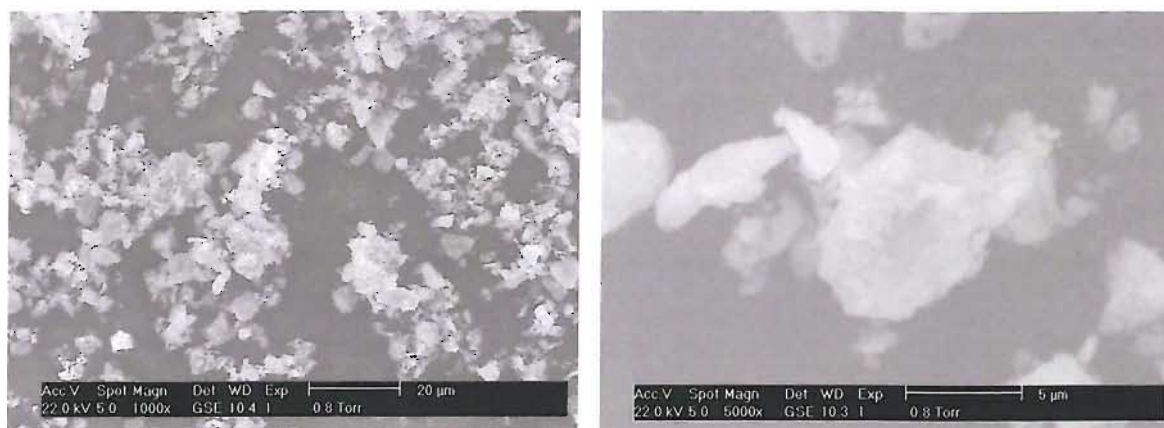
Fig. 4.3 SEM images of \text{LiFePO}_4 particles used for positive electrode
