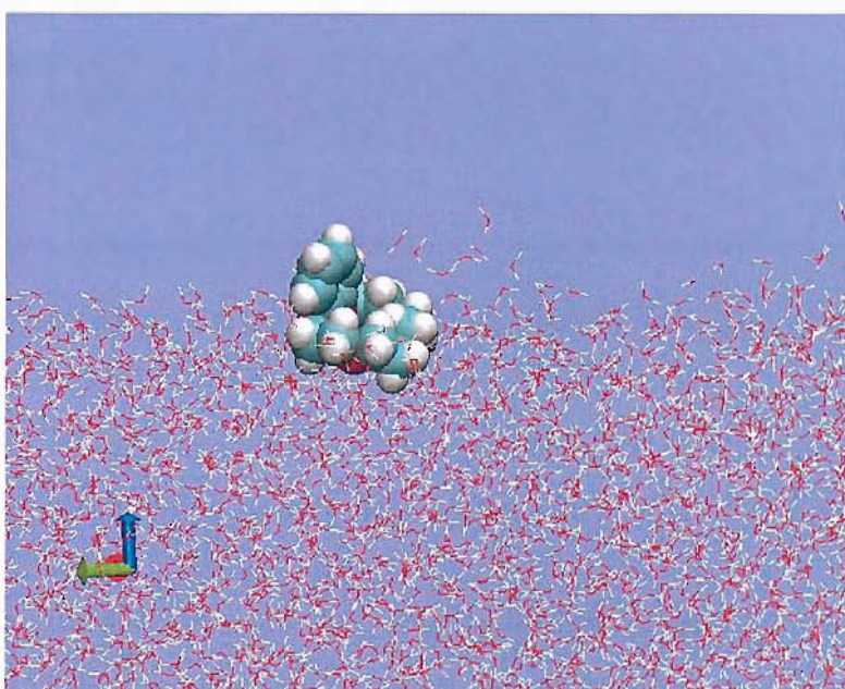
Figure 5.15: The straight conformation of benzo-15-crown-5 at the interface. This Figure shows a crown ether on the lower interface of the water layer. The red and white lines represent water molecules.
