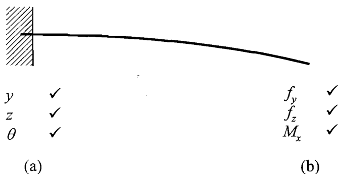
Figure 3.15: Cantilevered beam indicating which boundary values are known at each end (a) and (b)
