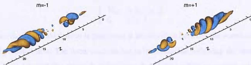
**Figure 3.24:** Response of the perturbed Rankine vortex, excited by a wavenumbers pair  $(m, k) = (1, 2\pi)$ . Iso-surfaces of radial velocity component:  $V_r = \pm 0.0004$ . Time=20.
