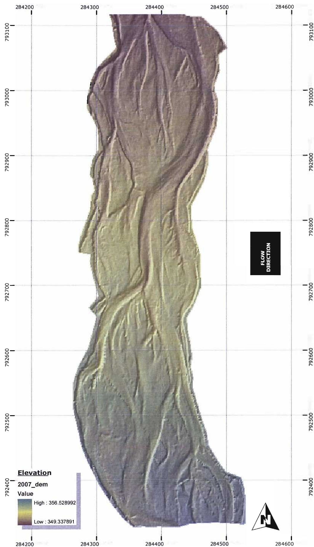
FIGURE C.9: 1 meter resolution DEM derived from 2007 GPS and total station survey.
