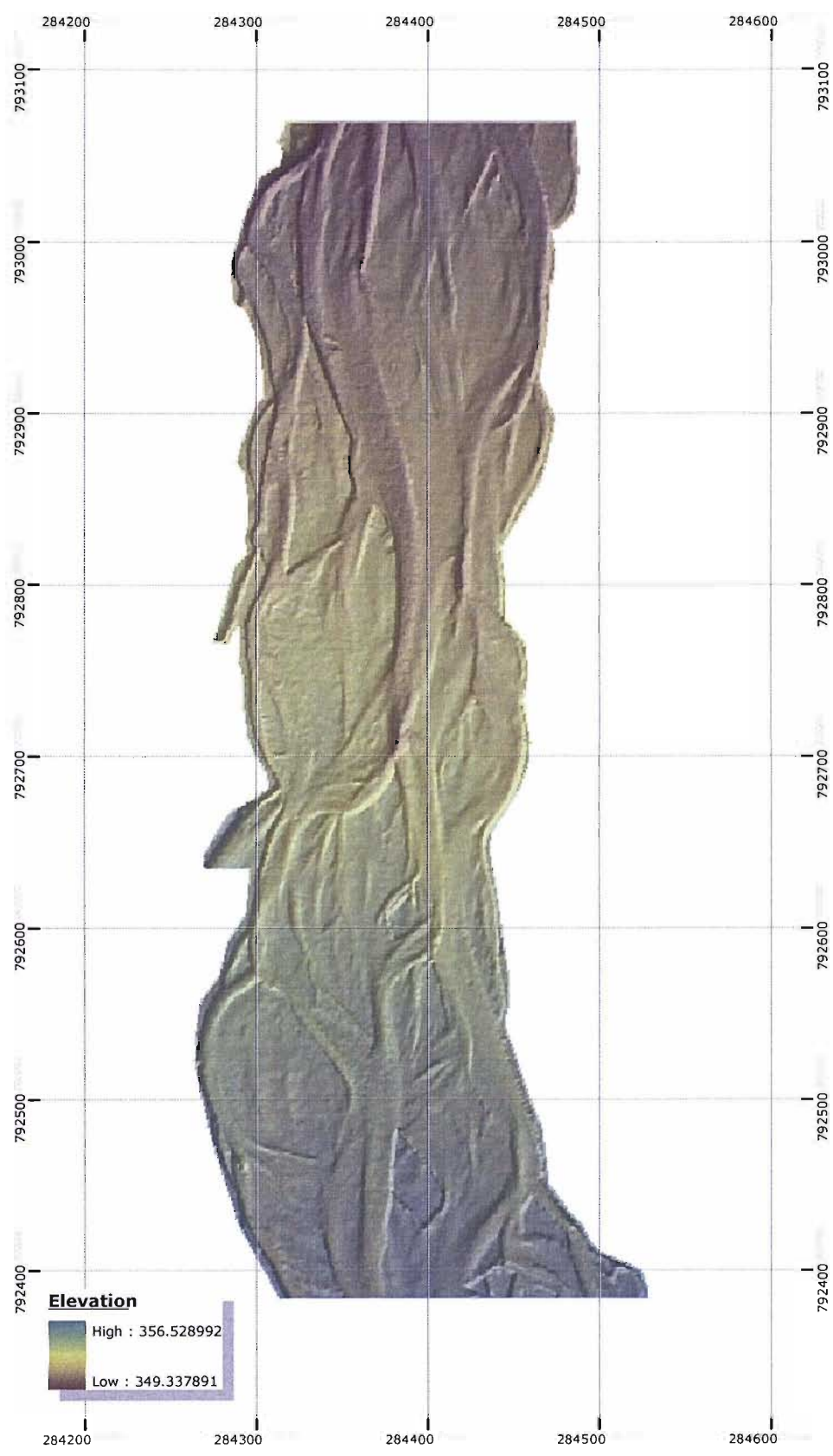
FIGURE C.6: 1 meter resolution DEM derived from 2004 GPS survey.
