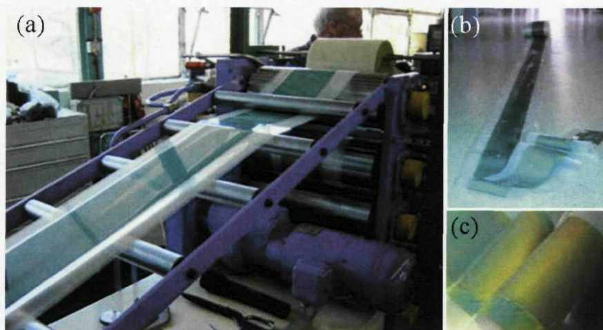
FIGURE 1.4: Polymer opals being manufactured in large quantities in (a) extrusion-to-roll manufacturing sequence. (b) Several meters of polymer opal sheet on a roll, with structural colour features in (c).
