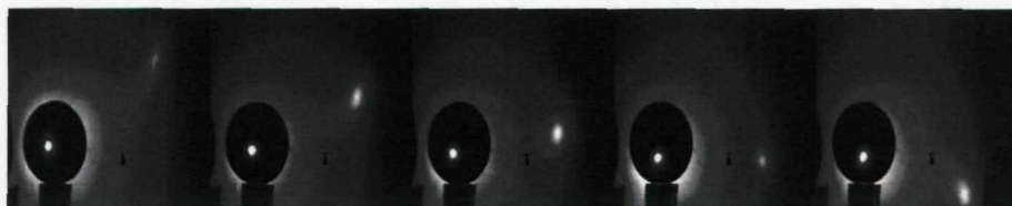
FIGURE 4.6: Evolution of the diffraction spot (bright spot on the right) around the reflected direction (bright spot on the left) with the changing angular position of the laser spot on the sample. Scan positions between \theta=40^\circ (left), \theta=-15^\circ (right).
